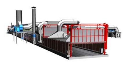
**Technofast** kiln is designed with an external supporting steel structure independent from the air **tight vapor fence** itself.
